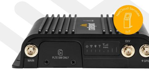
The R500-PLTE router with the Cradlepoint NetCloud Service for IoT is a purpose-built, low-cost User Equipment (UE) networking solution with industry-leading features for Private Cellular Networks (PCN). It is a compact, ruggedized solution for deployments in manufacturing, distribution, transportation, education, and others taking advantage of the lower fixed operating costs, enhanced data security, and improved network performance a PCN provides.
